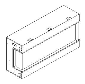
4. Remove the framing plates from the fireplace and fix them as the picture shows. NOTE: After removing the framing plates on the left and right sides, screw back the screws.
