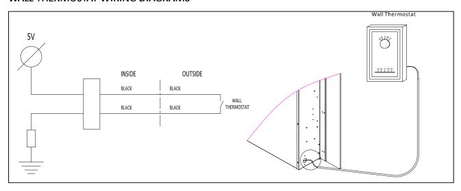
Wire the wall thermostat prior to installing the fireplace.
