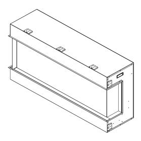
4. Remove the framing plates from the fireplace and fix them as the picture shows. NOTE: After removing framing plates on the left and right sides, screw back the screws.
