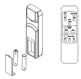
For remote to function make sure the heater is plugged in and main power switch located on the bottom left hand side is at position I.
