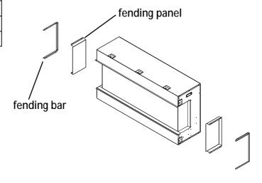
3. Screw back the fending bar after the panel is removed.
