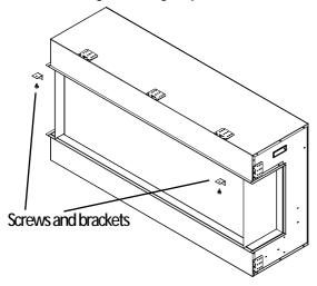
2. After the brackets are removed, the front glass panel will fall down automatically.
