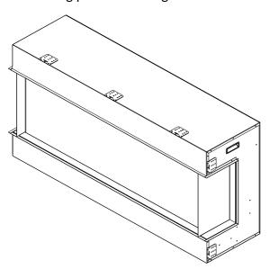
2. Unscrew 7screws on the right side that fix the fending bar and panel and then take off the fending bar and panel.
