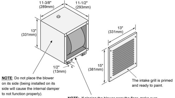
NOTE: If placing the blower near the floor, make sure the bottom edge is a min. 1-1/2" (39mm) above the finished floor to allow the grill to install.
