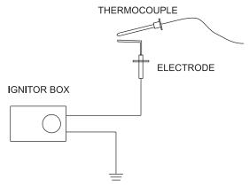
Figure 34 - Electronic Ignitor System Wiring
