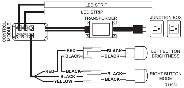
Figure 33 - LED System Wiring
