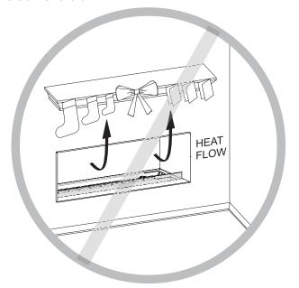
The flow of heat can ignite combustibles. For see-thru fireplaces, this applies to both sides of the
