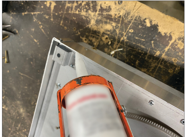
Figure 2.8, Silicone Rear of #HTK-EXT
