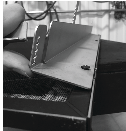
Figure 4.10, Screw Location on Hanging Bracket
