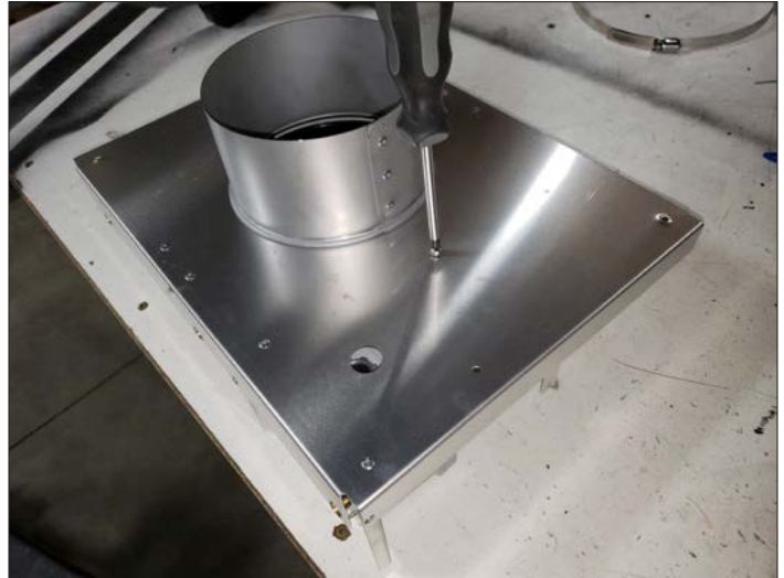
Figure 2.5, Remove (2) Screws on Backside of Assembly
