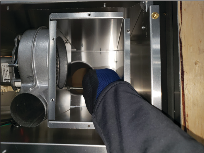
Figure 5.6, Remove (3) Screws Securing Fan Assembly
