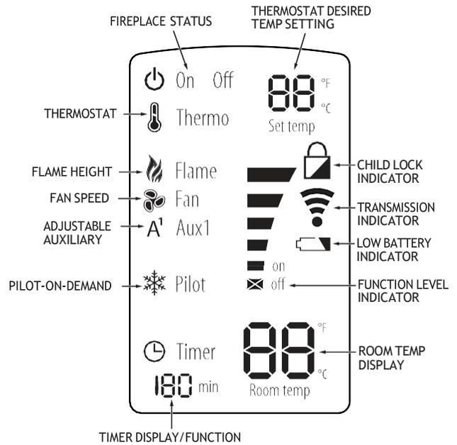
Figure 11.2, Komfort 8K Remote Control and Remote Control Display
