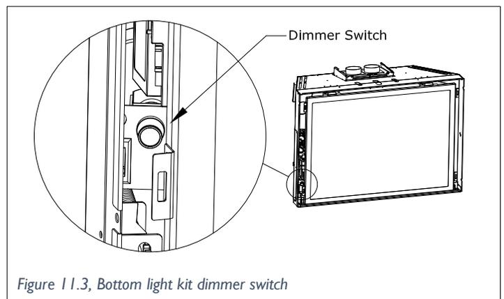
Figure 11.3, Bottom light kit dimmer switch
