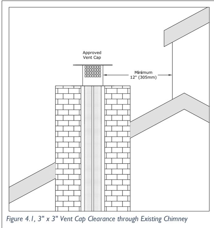
Figure 4.1, 3" x 3" Vent Cap Clearance through Existing Chimney
