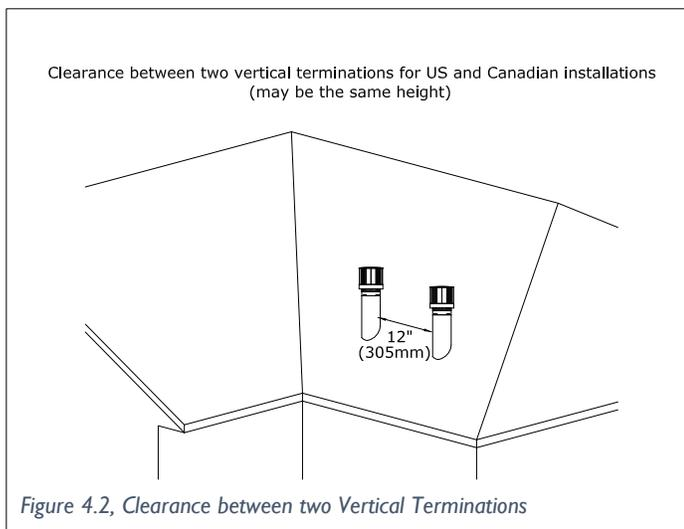
Figure 4.2, Clearance between two Vertical Terminations
