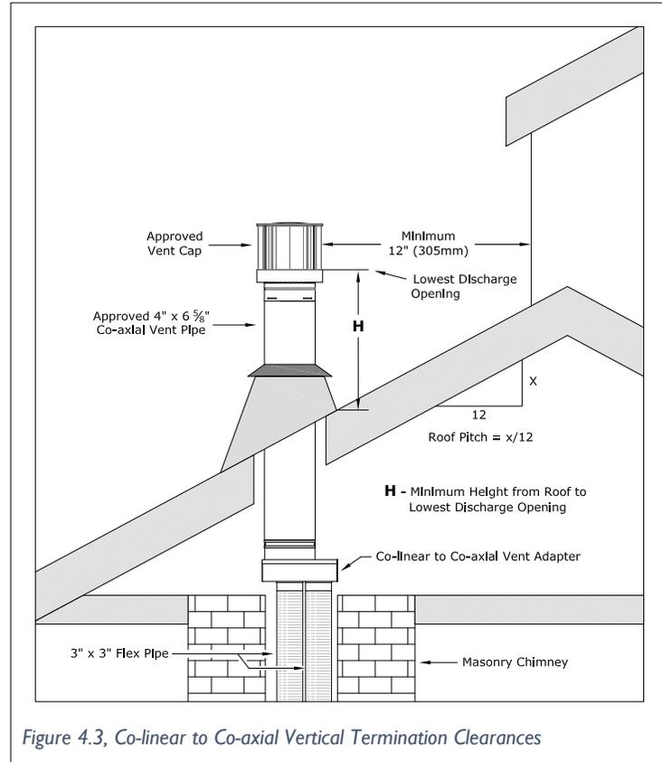
Figure 4.3, Co-linear to Co-axial Vertical Termination Clearances
