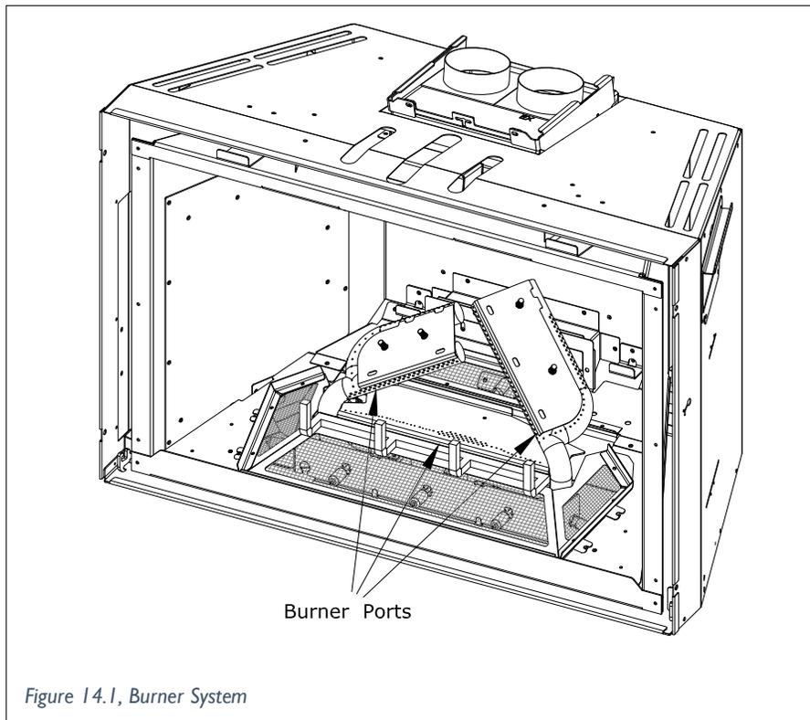
Figure 14.1, Burner System
