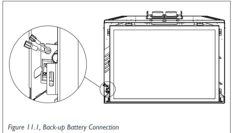
Figure 11.1, Back-up Battery Connection
