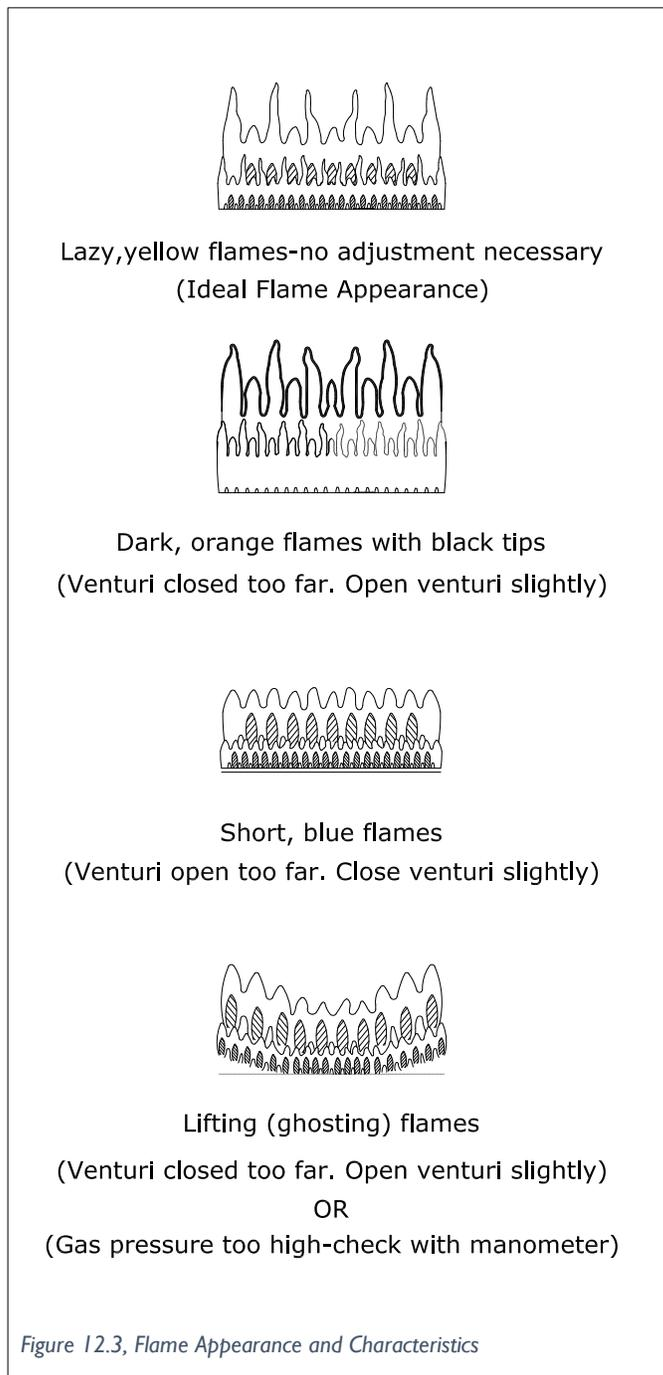
Figure 12.3, Flame Appearance and Characteristics
