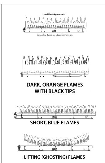
Figure 11.3, Flame Appearance and Characteristics
