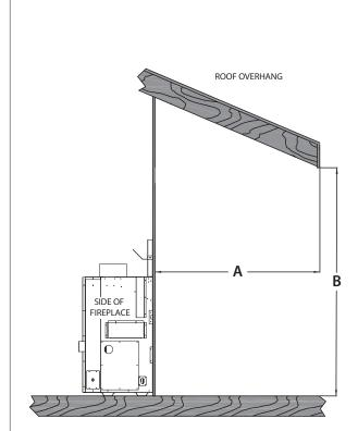
The overhang (A) must be a minimum of 1/2 or greater of the roofline elevation (B) above the base of the fireplace.
