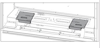
Figure 8.11. Control Board Removal and Installation - 1
