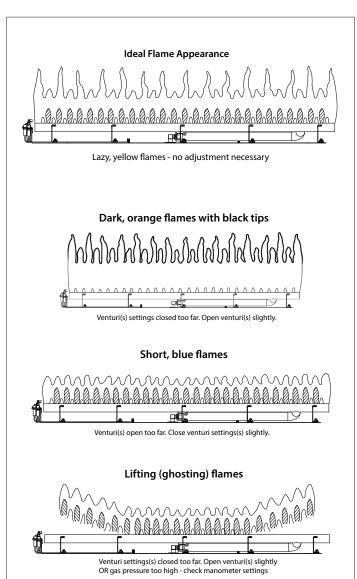
Figure 11.3, Flame Appearance and Characteristics
