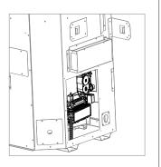
Figure 8.10, Control Board Access Cover
