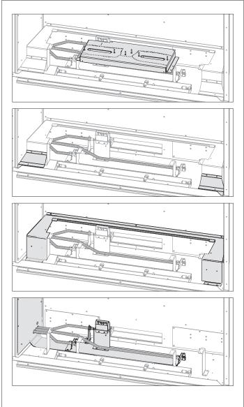
Figure 8.12, Control Board Removal and Installation - 2
