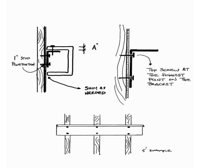
\*Picture below is if mantel is over metal on fireplace unit. Still finding 3 studs for 5ft and 4 studs for 6ft mantels.
