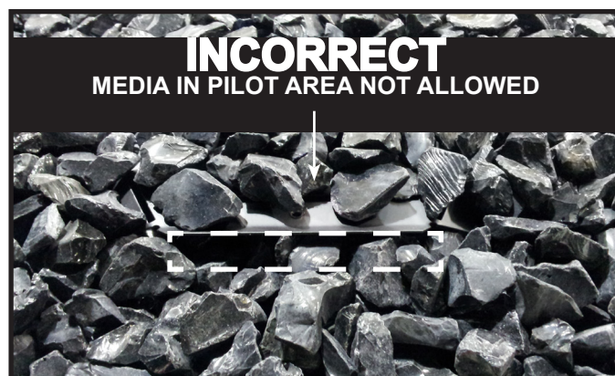
Figure 9.11 INCORRECT Media Placement
