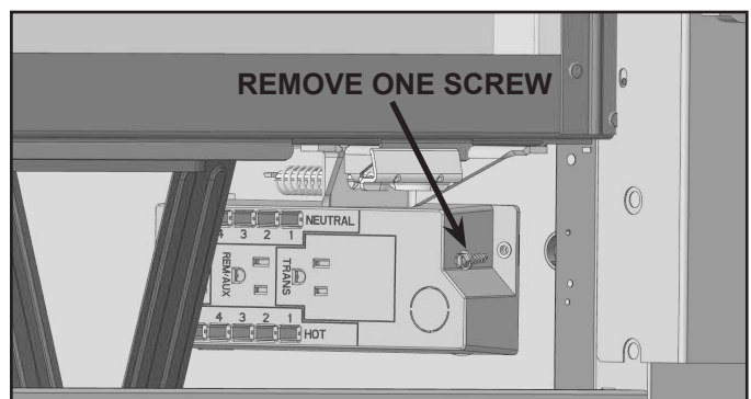
Figure 8.3 Junction Box Detail - JADE32IN-B
