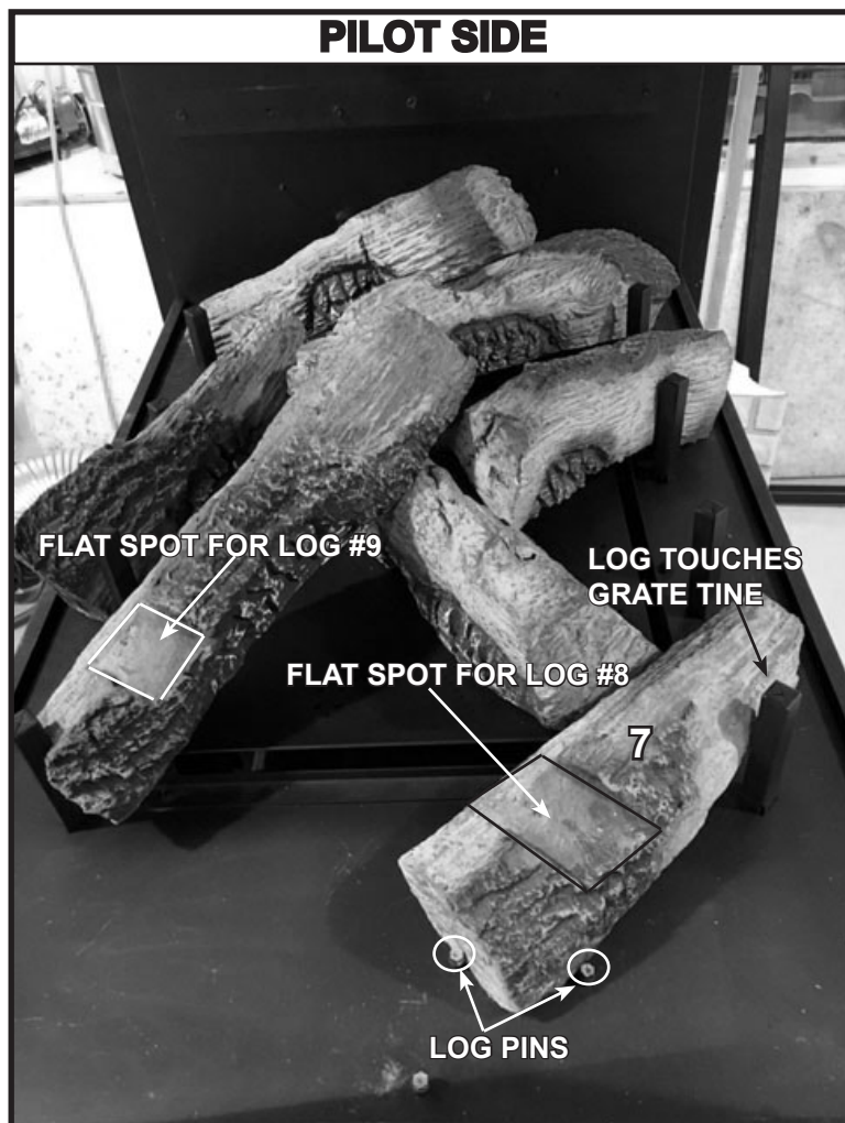
Figure 9. Log #7 Installed
