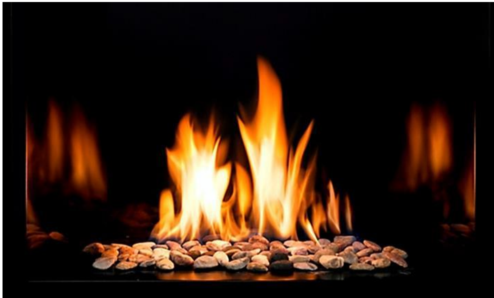
Figure 5-2 Burner Flame Heights: This image provides a visual reference for the burner flames burning at maximum height after the burners have been operating for 30 minutes or longer. A normal rear flame will be 1 to 2 inches above the rear log top edge. This, however, is dependent on the gas type, air shutter opening setting and vent system configuration. Actual flame heights can be slightly higher or lower when compared to this reference image.
