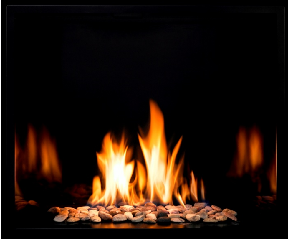
Figure 6-2 Burner Flame Heights: This image provides a visual reference for the burner flames burning at maximum height after the burners have been operating for 30 minutes or longer. This, however, is dependent on the gas type, air shutter opening setting and vent system configuration. Actual flame heights can be slightly higher or lower when compared to this reference image.
