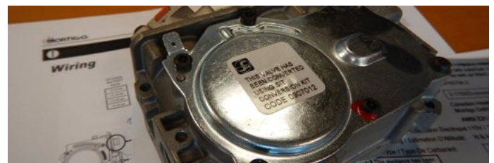
Figure 13.k Conversion label on valve
