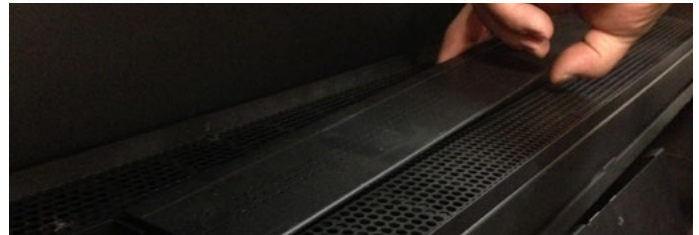
Figure 13.b Loosening the venturi
