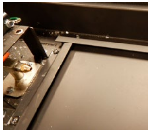
Figure 12.f Unscrewing brackets securing metal plate
