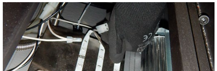
Figure 27.f Connect control board connector
