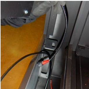
Figure 24.e On/Off switch through drawer
