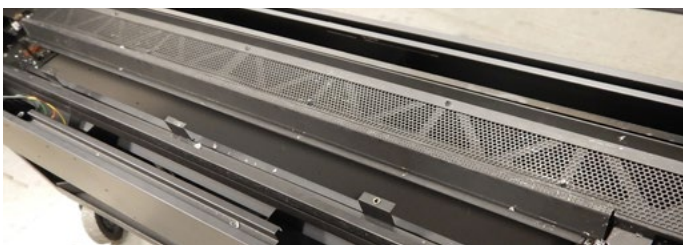
Figure 12.c Removing the media trays
