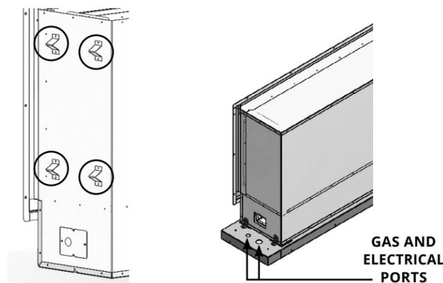
**3** Secure PART №9 Bracket (4) to fireplace and base using (8) ¼-20 x ½" long Pan Head Screws. Secure base to desired location with mounting holes and plum gas line thru and electrical lines thru the larger holes in the base
