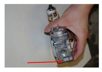
12) Place the Gas Valve into the machine vice using the provision as described above. Do not over tighten the vice. Remove the Flare Fitting from the gas outlet side of the valve.
