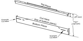
Reattach the top piece of the hearth trim to the cut bottom piece by fitting in place.
