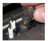
10) Unscrew the pilot orifice with the allen key; then replace with the LPG pilot orifice and the pilot cap, provided in the kit.
