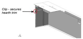
**6)** Line up the hearth trim with base of the unit and secure it with 3 screws as shown below.
