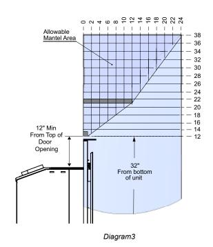
Note: A 3-1/2" mantel deflector to reduce mantel height to 32" from bottom of unit @ 1"depth.
