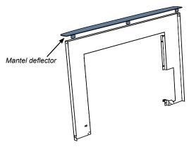
Bend all 3 tabs 90° to secure the deflector to the top of the backing plate.
