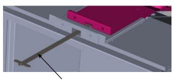
Flue Connector Slide Tool
