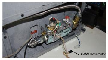
3) Disconnect the Cable coming from the Pressure Regulator Motor.
