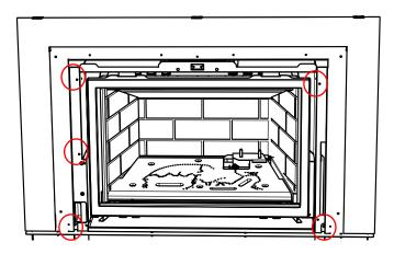
Separate the Outer Faceplate from the Backing Plate by removing 7 screws. 4. Install the mantel deflector in between the back of the outer faceplate and the front of the backing plate. Insert the screws from the front of the outer faceplate using 3 screws.
