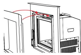
Hook onto unit to install
