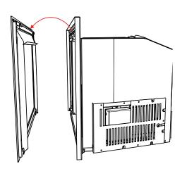
Remove 4 screws from the back of the Vignette faceplate in locations shown below—to remove the safety screen assembly.
