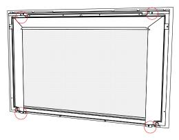
Remove 4 screws to remove safety screen assembly
