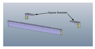
4) Attach the top and bottom part of the spacer brackets and then attach these spacer brackets to the assembled hearth trim with 3 screws.
