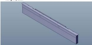
**4.** Line up the hearth trim with base of the unit and secure it with 3 screws as shown below.
