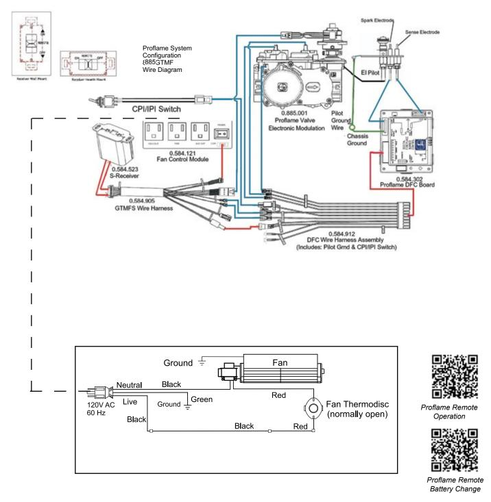
**GTMF REMOTE SYSTEM - IMPORTANT:** The 120V fan control module serves as the power source for this unit. The AA batteries in the receiver only serve as a backup in case 120 volt power lost within the home.
