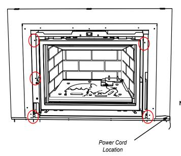
Install the Vignette faceplate by hooking the flange over the hanger as shown.
