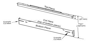
3) Similar to the front hearth trim, cut the top of the bottom piece of the spacer brackets to the appropriate height.
