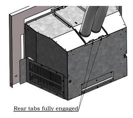
Properly installed Flue Connector Plate
