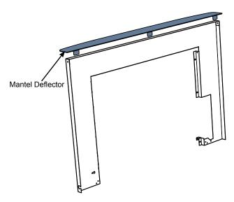
2. Bend all 3 tabs 90° to secure the deflector to the top of the backing plate. The tabs should be flush with the underside of the top lip of the back plate.
