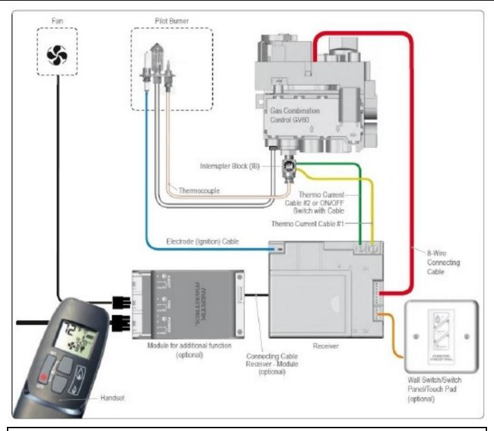
**Caution:** Label all wires prior to disconnection when servicing the controls. Wiring errors can cause improper and dangerous operation. Verify proper operation after servicing.
