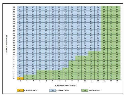
Power vent runs of up to 110ft with (6) 90° elbows are permitted when using the SOLAS power vent kit PV-486072. Refer to power vent instructions for additional power vent installation and operation information.
