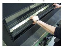
2. Remove the left and right side panels by lifting up and toward you.
