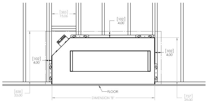
Sometimes it is necessary to frame the location you will be installing the fireplace before the fireplace is onsite, the above image shows an example of how to frame the wall before the fireplace is moved into position.
