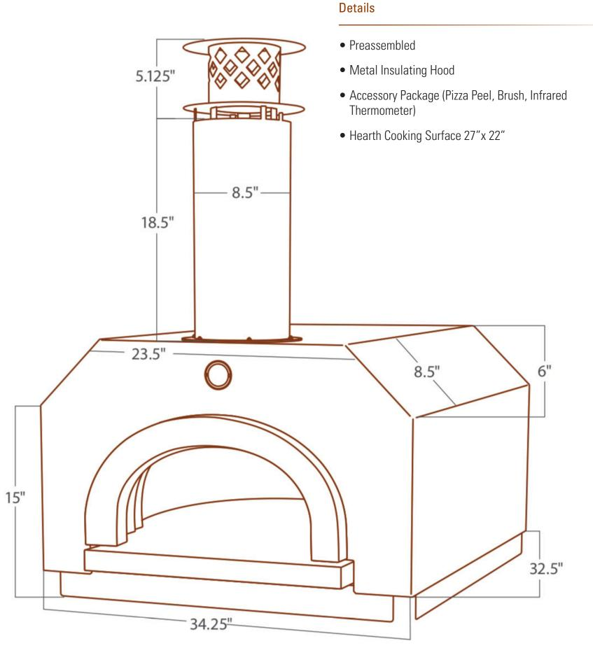
Minimum Support Weight: 450 lbs. Flue Pipe Dimensions: 27.25" H x 22.25" W
