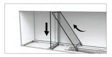
10. Insert the full height glass panel into one of the open end side by inserting the glass into the opening at the top of the appliance, and lowering it into the slots in the base until it bottoms out into place. Repeat the same for the other side of the appliance.
