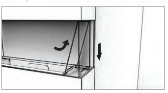
10. Install the windscreen by inserting the glass ends into the slots. Use a small amount of pressure to push the windscreen in place until it bottoms out into the hidden glass clips.
