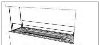
10. If your appliance includes a decorative box on the left / right or both, insert the internal glass panel by feeding the glass upwards into the slot then pushing down into the positioned clips.
