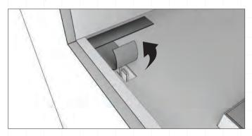
9. Install the windscreen by inserting the two ends into appropriate slots in the appliance. Use a small amount of pressure to push the windscreen in place until it bottoms out into the hidden glass clips. Repeat the same for the back side windscreen and if your appliance includes a decorative box on the left / right or both.
