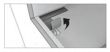
10. If your appliance includes a decorative box on the left / right or both, insert the internal glass panel by feeding the glass upwards into the slot then pushing down into the positioned clips.
