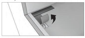
9. If your appliance includes a decorative box on the left / right or both, insert the internal glass panel by feeding the glass upwards into the slot then pushing down into the positioned clips.
