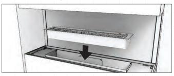
8. Remove the dust protective tape that covers the windscreen mounting slots.
