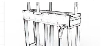
3. Slide the appliance inside the framing cavity (the bottom tray can sit directly on top of the frame). The appliance is shipped with red stability bracket(s) installed on the open side(s) to keep the appliance square while in transport and during installation. Keep the bracket(s) on while framing up the setting to assist in minimising movement of the appliance.
