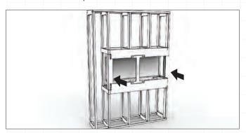
3. Secure the appliance to the framework using the existing mounting holes on the appliance flanges. Make sure that the appliance is level before securing it in place.
