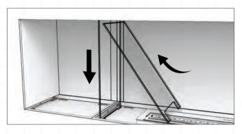
11. Install the windscreen by inserting the two ends into appropriate slots in the appliance. Use a small amount of pressure to push the windscreen in place until it bottoms out into the hidden glass clips. Repeat the same for the back side windscreen.
