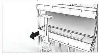
Complete the construction by finishing the wall paneling around the appliance. (See section on FINISHING INSTRUCTIONS and ensure that you fully understand where non combustible materials must be used.)
