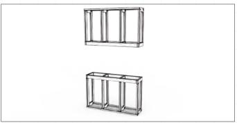
ch will assist in leveling appliance. Screw it into place using the included screws (bottom row onto appliance, top row onto framing material) to secure it into position.
