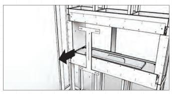
7. Complete the construction by finishing the wall paneling around the appliance. (See section on FINISHING INSTRUCTIONS and ensure that you fully understand where non combustible materials must be used.)
