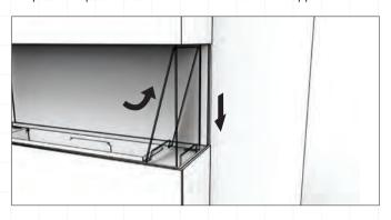
11. Install the windscreen by inserting the two ends into appropriate slots in the appliance. Use a small amount of pressure to push the windscreen in place until it bottoms out into the hidden glass clips.
