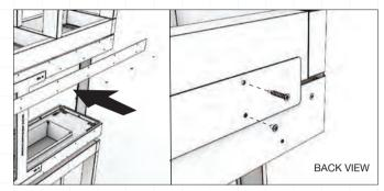
Remove the extension flange from the fireplace so that both sides are the same height. This will help make sliding the fireplace into the frame easier. Pay attention not to lose the screws, they will be needed again when the flange is re-installed.
