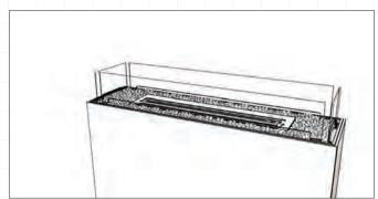
8. Remove the dust protective tape that covers the windscreen mounting slots.
