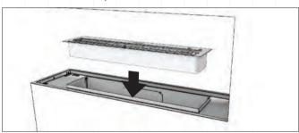
12. Install the windscreen by inserting the two ends into appropriate slots in the appliance. Use a small amount of pressure to push the windscreen in place until it bottoms out into the hidden glass clips. Repeat the same for the back side windscreen.
