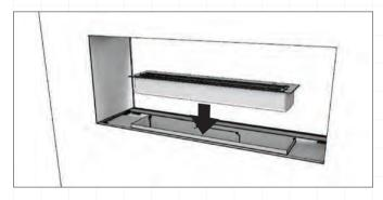
9. Remove the dust protective tape that covers the windscreen mounting slots.
