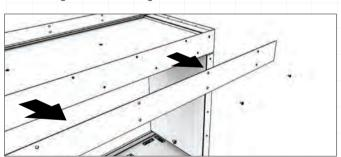
5. Fix the appliance to the framework with screws using the existing mounting holes on the appliance flanges. Make sure that the appliance is level before securing it in place.
