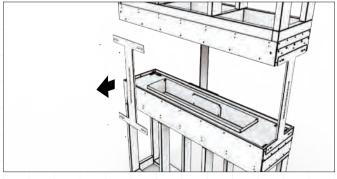
7. Complete the construction by finishing the wall paneling around the appliance. (See section on FINISHING INSTRUCTIONS and ensure that you fully understand where non combustible materials must be
