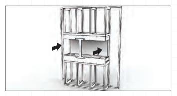
Ensure that the left and right side edges of the appliance are flush to the frame-work studs.
