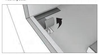
10. Install the windscreen by inserting the two ends into appropriate slots in the appliance. Use a small amount of pressure to push the windscreen in place until it bottoms out into the hidden glass clips. Repeat the same for the back side windscreen and if your appliance includes a decorative box on the left / right or both.
