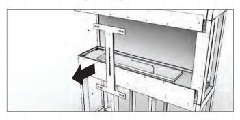
Complete the construction by finishing the wall paneling around the appliance. (See section on FINISHING INSTRUCTIONS and ensure that you fully understand where non combustible materials must be used.)
