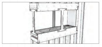
4. Align the flange extension panel with the threaded holes on the appliance. Screw it into place using the included screws (bottom row onto appliance, top row onto framing material) to secure it into position.
