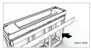
Remove the extension flange from the firebox so that both sides are the same height. This will help make sliding the firebox into the frame easier. Pay attention not to lose the screws, they will be needed again when the flange is re-installed. Fix the appliance to the framework with screws using the existing mounting holes on the appliance flanges. Make sure that the appliance is level before securing it in place.
