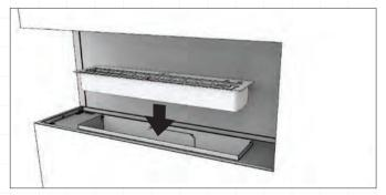
7. Remove the dust protective tape that covers the windscreen mounting slots.
