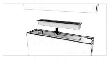
9. Remove the dust protective tape that covers the windscreen mounting slots.
