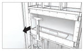
Complete the construction by finishing the wall paneling around the appliance. (See section on FINISHING INSTRUCTIONS and ensure that you fully understand where non combustible materials must be used.)
