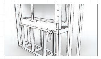
2. Slide the appliance inside the framing cavity (the base of the appliance can sit directly on top of the 2 x 4 framing material). The appliance is shipped with red stability bracket(s) installed on the open side(s) to keep the appliance square while in transport and during installation. Keep the bracket(s) on while framing up the setting to assist in minimizing movement of the appliance.
