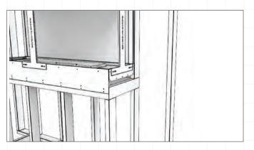
4. Secure the appliance to the framework with screws using the existing mounting holes on the appliance flanges. Make sure that the appliance is level before securing it in place.
