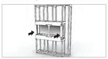
Secure the appliance to the framework using the existing mounting holes on the appliance flanges. Make sure that the appliance is level before securing it in place.
