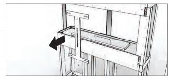
7. Complete the construction by finishing the wall paneling around the appliance. (See section on FINISHING INSTRUCTIONS and ensure that you fully understand where non combustible materials must be used.)
