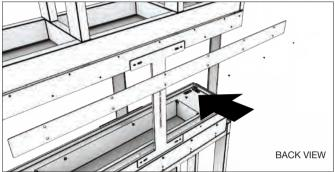
4. Align the flange extension panel with the threaded holes on the
