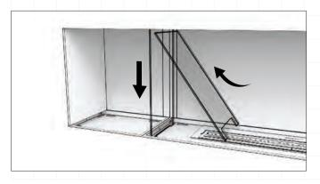
9. Install the windscreen by inserting the two ends into the appropriate slots in the appliance. Use a small amount of pressure to push the windscreen in place until it bottoms out into the hidden glass clips.
