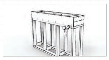
3. Slide the appliance inside the framing cavity (the bottom tray can sit directly on top of the frame).
