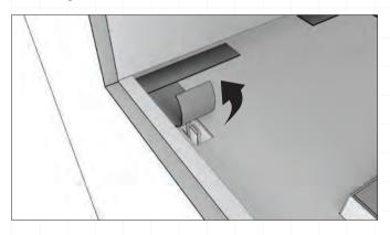
8. If your appliance includes a decorative box on the left / right or both, insert the internal glass panel/s by feeding the glass upwards into the slot then pushing down into the positioned clips.
