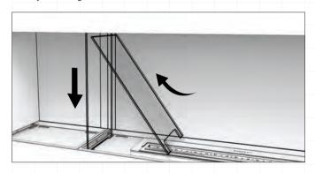
9. Insert the full height glass panel into one of the open end side by inserting the glass into the opening at the top of the appliance, and lowering it into the slots in the base until it bottoms out into place.
