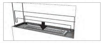
9. Remove the dust protective tape that covers the windscreen mounting slots.
