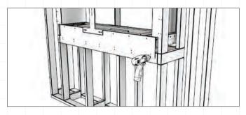
3. Slide the appliance inside the framing cavity (the bottom tray can sit directly on top of the frame). The appliance is shipped with red stability bracket(s) installed on the open side(s) to keep the appliance square while in transport and during installation. Keep the bracket(s) on while framing up the setting to assist in minimising movement of the appliance.
