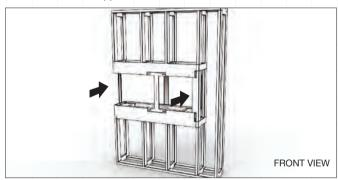
3. Ensure that the back and open side edge of the appliance **are flush** with frame studs.
