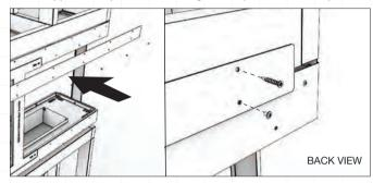
5. Fix the appliance to the framework with screws using the existing mounting holes on the appliance flanges. Make sure that the appliance is level before securing it in place.
