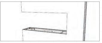
11. Insert the full height glass panel into the open end side by inserting the glass into the opening at the top of the appliance, and lowering it into the slots in the base until it bottoms out into place.
