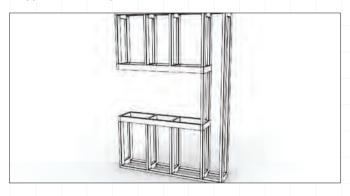
2. Slide the appliance into the framing cavity (the bottom tray can sit directly on top of the frame). The appliance is shipped with red stability bracket(s) on the open sides to keep the appliance square while in transport and during installation. Keep these brackets on while framing up the setting to assist in minimizing movement of the appliance.
