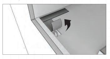
8. If your appliance includes a decorative box on the left / right or both, insert the internal glass panel by feeding the glass upwards into the slot then pushing down into the positioned clips.
