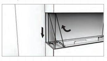
10. Install the windscreen by inserting the glass ends into the slots. Use a small amount of pressure to push the windscreen in place until it bottoms out into the hidden glass clips.
