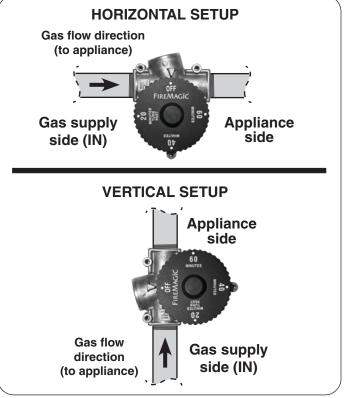
Fig. 1-2 Automatic timer shut-off valve installation detail
