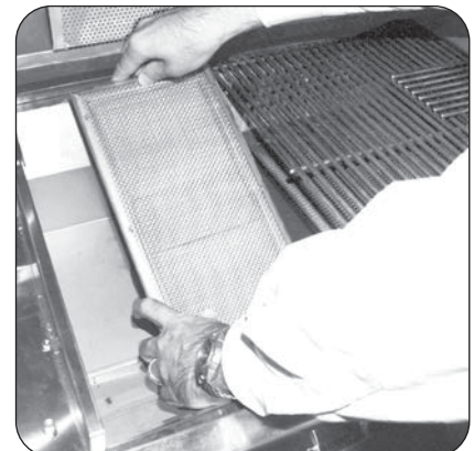
Fig. 3-5 Install new burner
