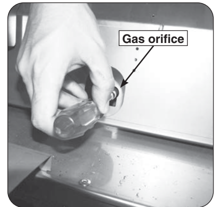
Fig. 3-2 Replace the gas orifice
