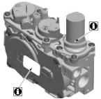
This heater is either approved for natural gas (NG) or for propane (LP). Burning the incorrect fuel will void the warranty and safety listing and may cause an extreme safety hazard. Direct questions about the type of fuel used to your dealer. Check for a label on the flame adjust knob on the gas control valve (this is the best place to check). You may also check for a label on the gas control valve body.
