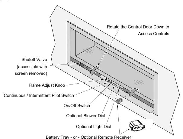
On/Off Switch This control is used to turn the heater on and off.
