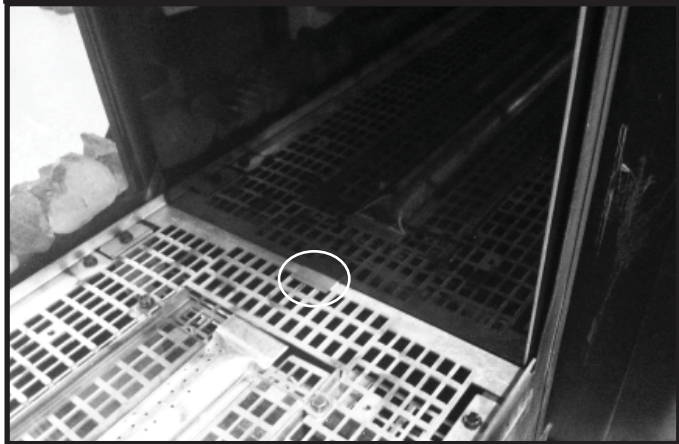
Figure 10.8 Position Glass Clip and Install Glass Panel
