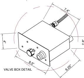
SPARK IGNITION BY AA BATTERY MATERIAL: 304 STAINLESS STEEL
