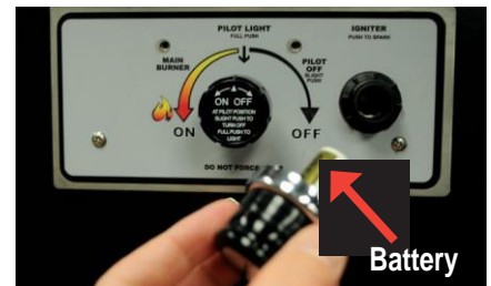
Figure 10.6 – Slide battery into spark igniter unit.
