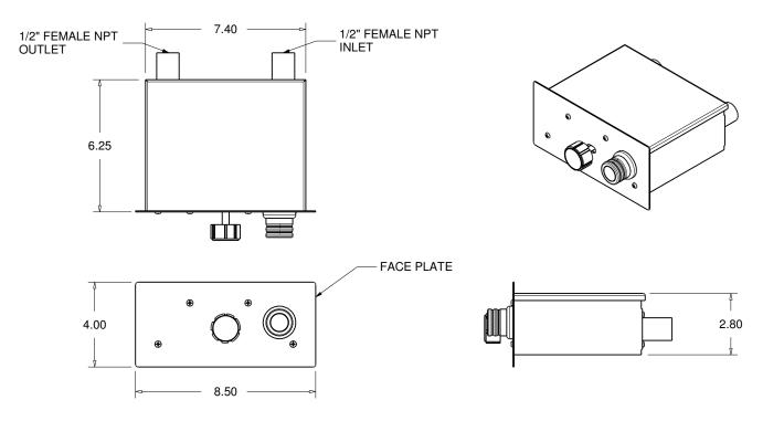
SPARK IGNITION BY AA BATTERY MATERIAL: 304 STAINLESS STEEL
