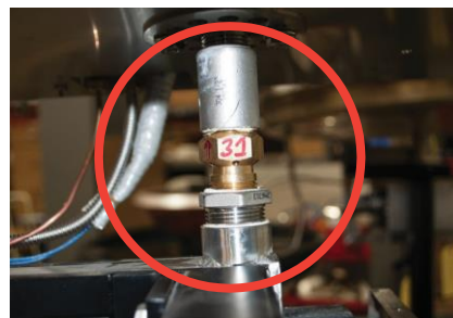
Figure 9.1 – Locating orifice for cleaning
