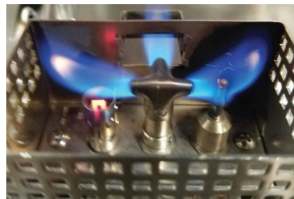
Figure 9.2 – Pilot flame coverage of thermocouple.
