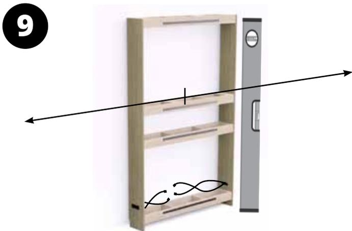
Locate center of main unit and align with previously marked center.
