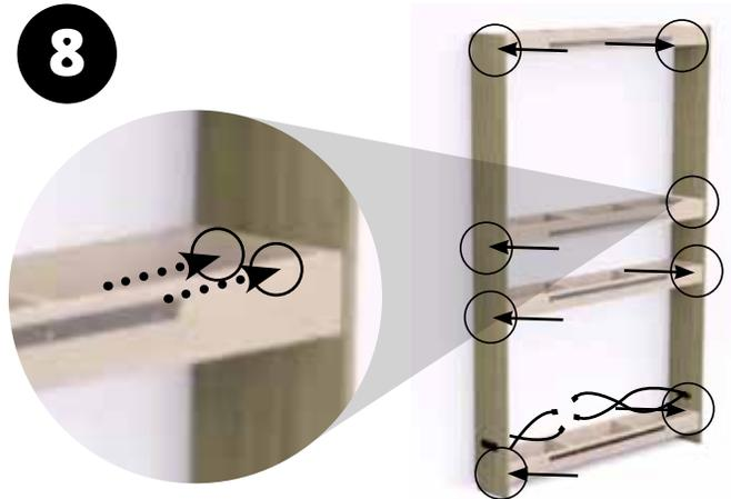
Raise wall. From the bottom of unit, remove & reuse previous screws, see step 5, and add second secure screws sixteen (16), making sure to keep wall flush with side wall upright.
