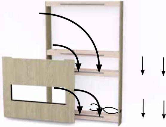
Mount fireplace front facia, by sliding onto attached upper and lower horizontal mounting strips secured to wall unit.
