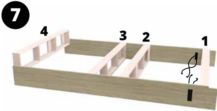
...then screw into side wall until flush with inner box frame.
