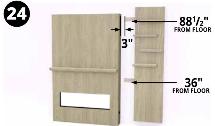
Once cleat mounts are measured, leveled and secure, lift the shelf wall with secured shelves and place over the cleat mounts
