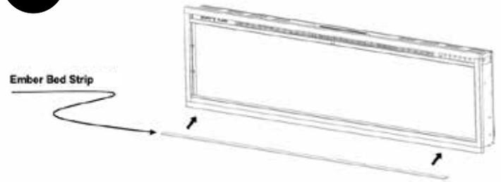
Place the ember bed strip in position, if ember bed strip is not factory installed.
