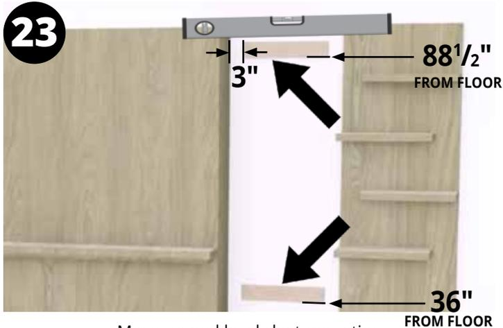
Measure and level cleat mounting (wood) brackets. Cleat mount brackets MUST attach to at least one (1) stud in wall. Use at least two (2) screws into wall.
