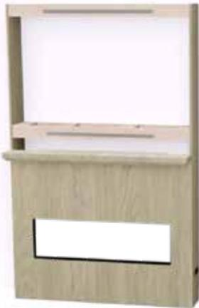
Place mantel in mount, in lower guide, then prepare for upper front facia. No screws needed, mantel will be secured by lower & upper facia.
