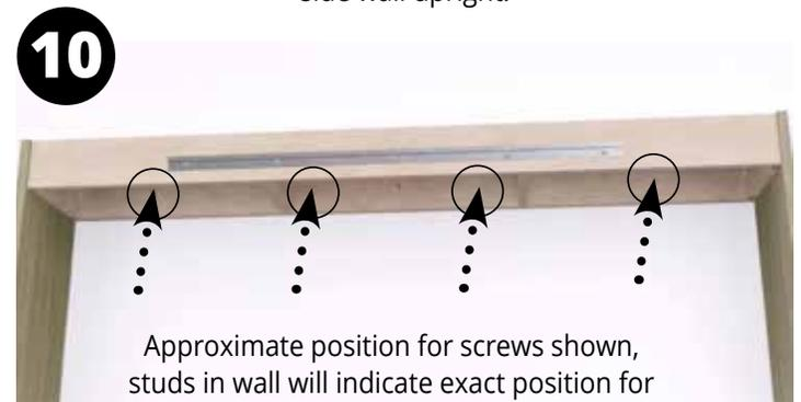
Approximate position for screws shown, studs in wall will indicate exact position for securing screws
