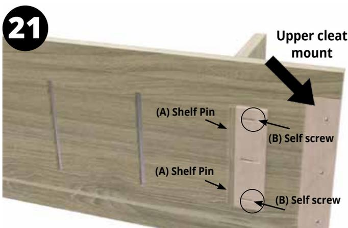
Once shelf is in place and desired position, then place (A) shelf pins to secure shelves temporarily. Then (B) insert and tighten shelf screws.
