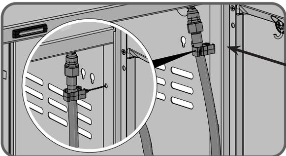
**WARNING!** Clip hose to side cart panel using bushing supplied. Failure to follow these instructions could result in property damage, personal injury or death.
