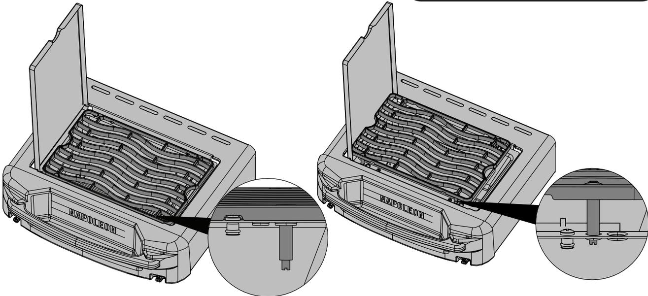
**Cooking Grid Placement:** The cooking grid can be placed at two different heights. The lower height is for use with pots or pans. The higher position is to be used when searing meats. Ensure the burner is off and the grid is cool to the touch before changing between the two heights. The grid must be at the lower height in order to close the lid.
