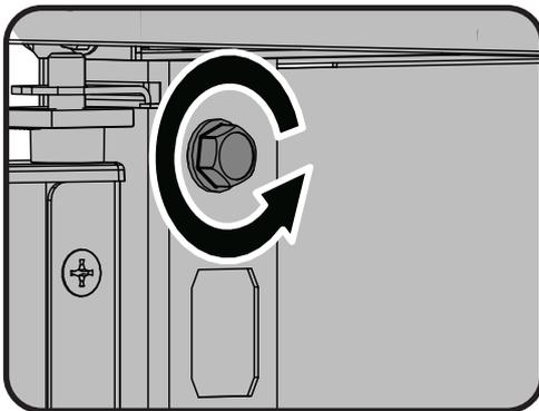
The depth of the door leveling screw will adjust the fit of the doors.
