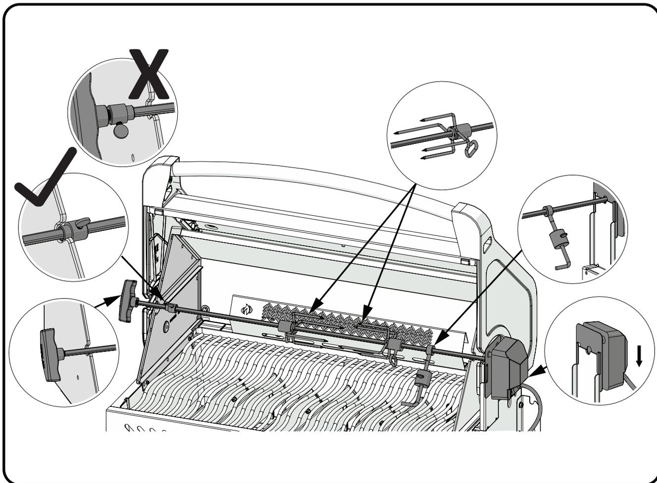
**Ensure stop bushing is tightened on the inside of hood casting.**
