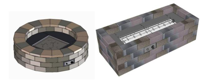
With gas hookups completed and burner installed, install remaining layers of block and secure with construction adhesive .
