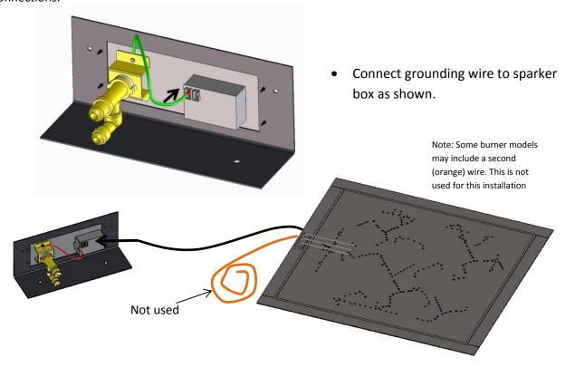
• Plug the **black** sparker wire into the igniter box. <u>A sparker wire extender is included in your kit if the burner's wire does not reach your control panel location.</u>
