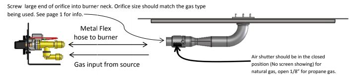
When hooking up gas to burner, be sure to turn off gas flow at the source (by closing valve on propane tank or natural gas line) before making any connections. Tighten all gas connections securely using two wrenches
