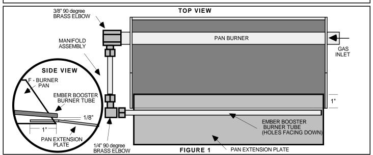
**OPERATION:** Flame should burn evenly across both burners. If not, the sand may not be completely covering the Ember Booster Burner and/or the Pan Burner. **Sand must completely cover both burners!** Also, sand may have become packed during installation of the Ember Booster Burner. Using a kitchen knife, putty knife or spatula, loosen the sand by inserting knife edge under the embers. Loosen the entire bed and recheck for even distribution of ember material and flame.
