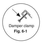
4. Should the damper clamp not fit, install a permanent damper stop or provide some other means of preventing full and/or accidental closure of the damper such as removing the damper blade.
