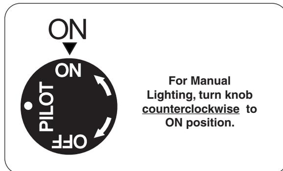
Fig. 27-1 Control knob detail (ON)
