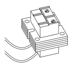
Figure 1. A 24 VAC 20 VA Class 2 Transformer with a UL/CSA listing is required for each heater. Transformer is to be supplied by installer
