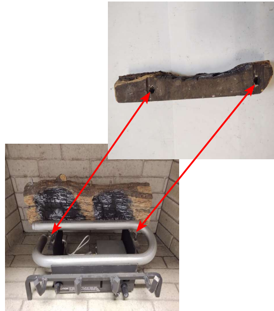
Figure Q - Middle Log Placement
