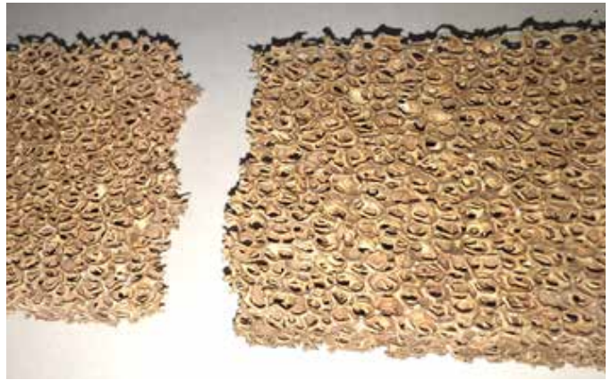
Combustor Problem - Broken Combustor
