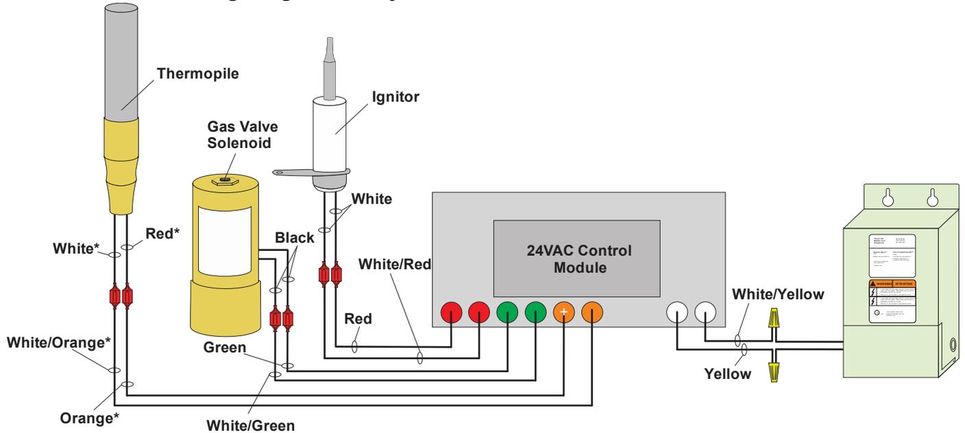
\* **NOTE:** The thermopile must connect to the control module as shown above (**white/orange** wire connects to the **white** thermopile wire and **orange** wire connects to **red** thermopile wire). **Do not reverse the wires.** If the wires are reversed, the Lantern will not work correctly.
