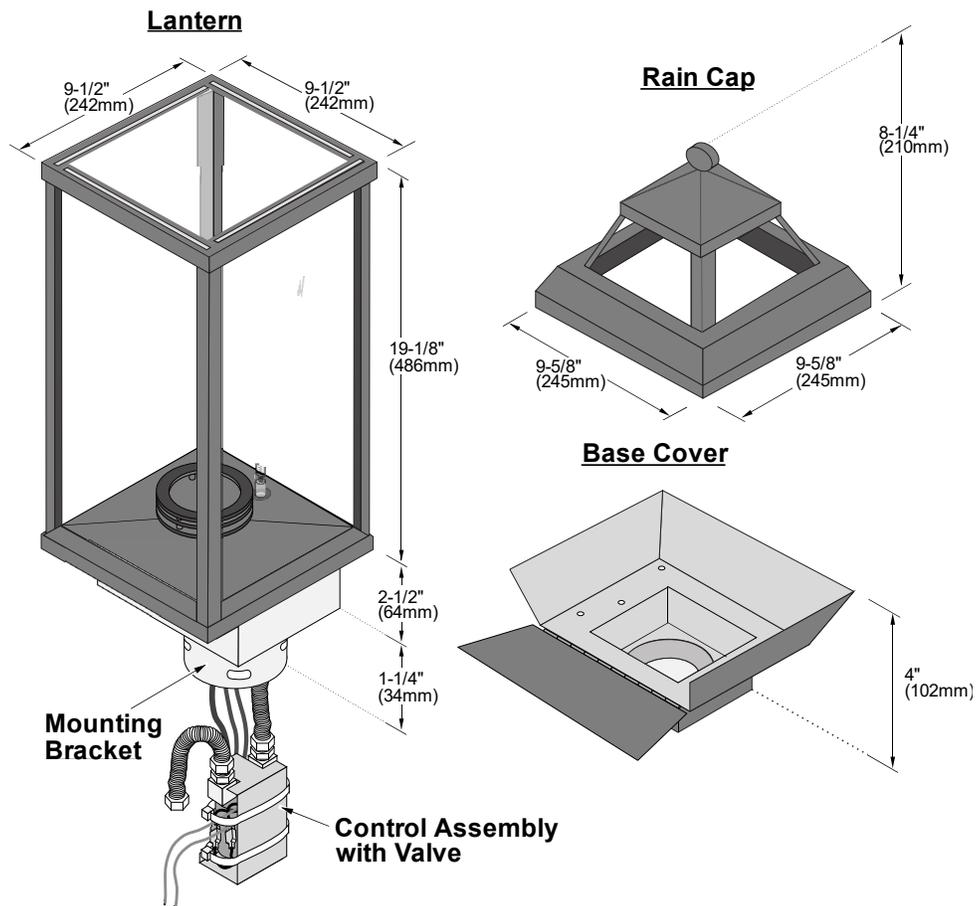
**NOTE:** Side clearances are measured from the glass – Top clearances are measured from the glass frame.
