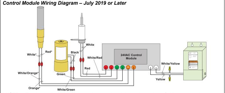
\* NOTE: The thermopile must connect to the control module as shown above (white/orange wire connects to the white thermopile wire and orange wire connects to red thermopile wire).
