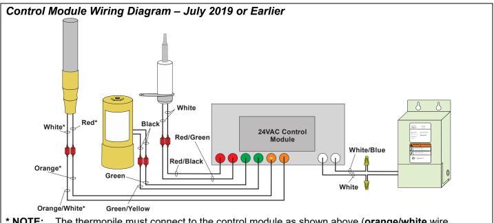
\* NOTE: The thermopile must connect to the control module as shown above (orange/white wire connects to the white thermopile wire and orange wire connects to red thermopile wire).
