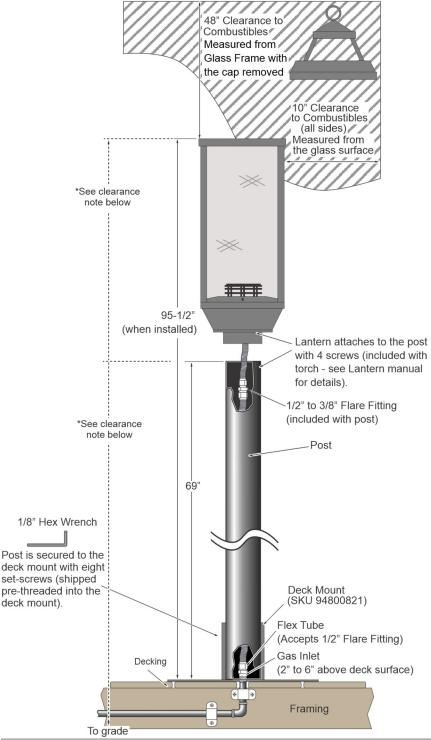
\*NOTE: The distance from ground level to the top of the Lantern shall be a minimum of 7' (2.1m) where installed within 2' (0.6M) of public walkways (e.g.: sidewalk, shared walkway between two homes, or pathway in commercial applications). Lesser clearances shall be permitted to be used only where acceptable to the authority having jurisdiction.
