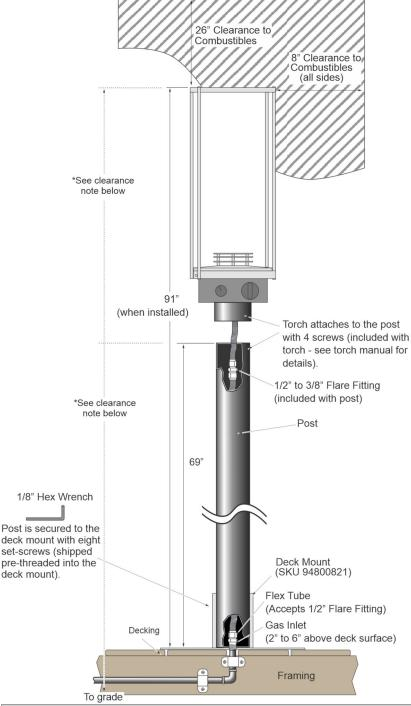
\*NOTE: The distance from ground level to the top of the Torch shall be a minimum of 7' (2.1m) where installed within 2' (0.6M) of public walkways (e.g.: sidewalk, shared walkway between two homes, or pathway in commercial applications). Lesser clearances shall be permitted to be used only where acceptable to the authority having jurisdiction.
