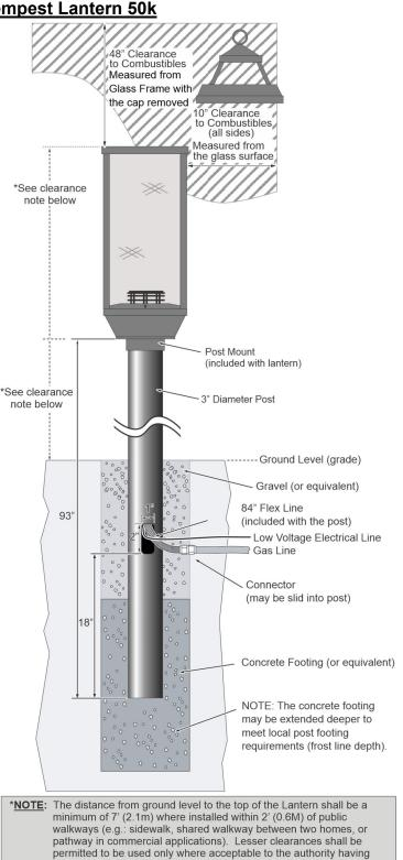
57-1/2" - Minimum height above grade the top of the post must be above grade to meet this requirement.
