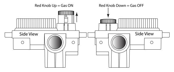
Fig. 5 E-Stop Gas Timer red knob positions
