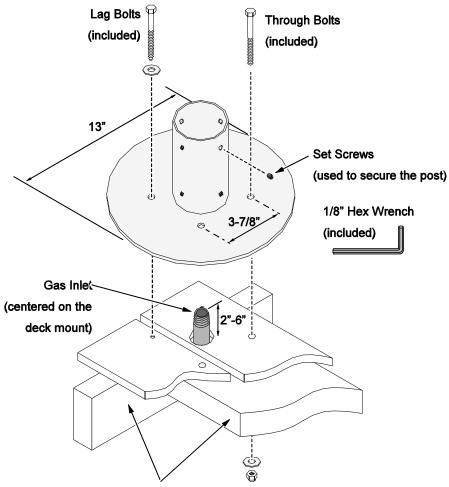
The post mount <u>must be secured to deck framing in four locations</u> (or other secure footing - the deck surface is not adequate for proper support).
